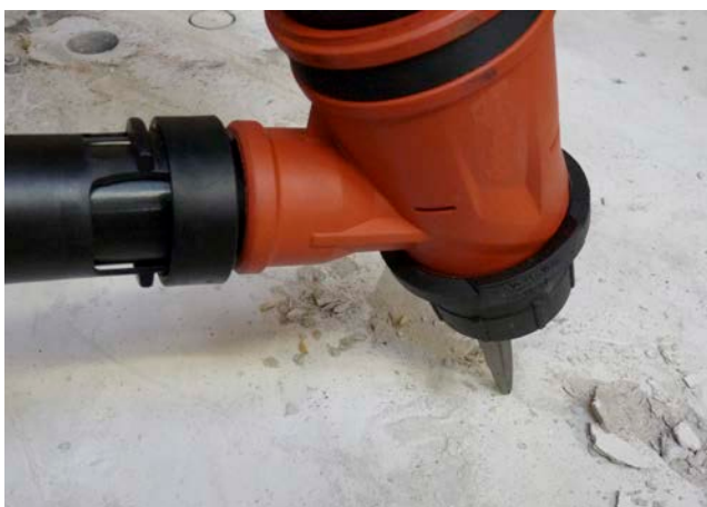
Figure 2 Examples of captor hoods on a grinder and breaker
