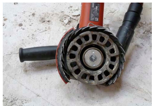
Figure 1 Tools and accessories providing for effective dust removal
