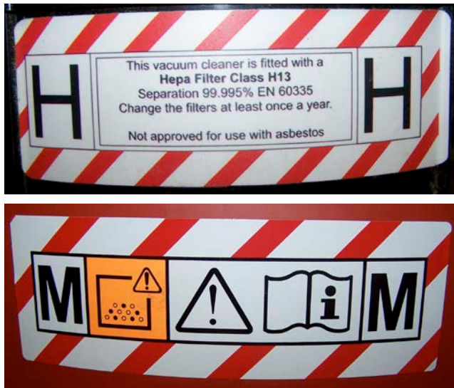
Figure 4 Examples of labels on H and M class extraction units
