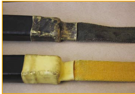
Figure 5 Two similar products with unknown history – the top webbing is heavily soiled
