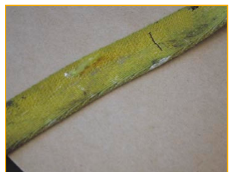
Figure 4 Surface fibres damaged by abrasion
