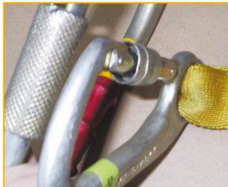
Figure 7 Damaged gate on karabiner
