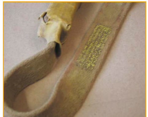
Figure 8 Missing label: damage to protective sleeve over energy absorber
