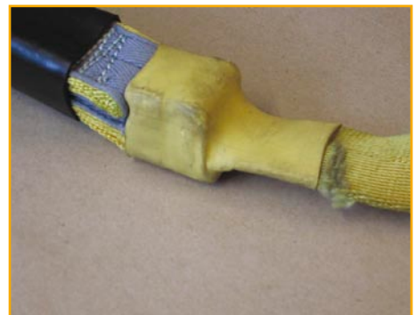
Figure 2 Abrasion damage adjacent to energy absorber: displaced protective sleeve over energy absorber
