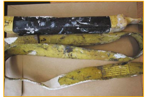
Figure 6 Heavy paint contamination to webbing
