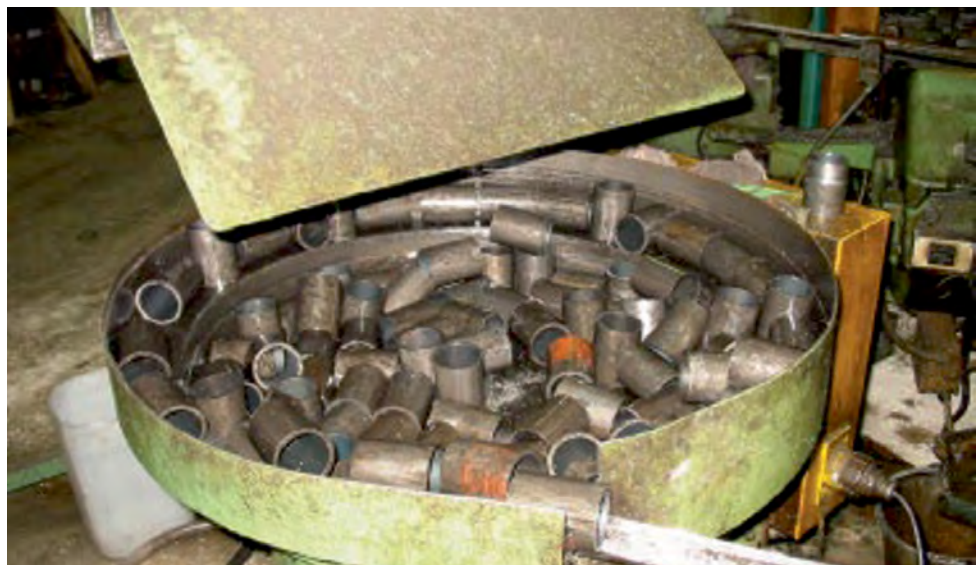
Figure 4 Reduced drop heights to reduce noise
