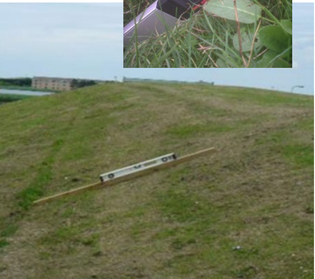
Consider using a straight edge in conjunction with slope measuring device when surveying longer spans
